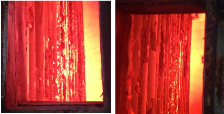
Before cleaning: Extensive scale, hot spots, pieces of refractory
